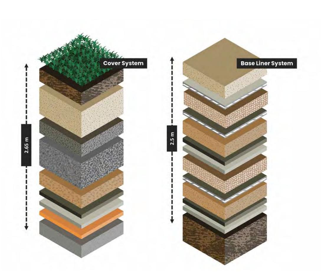
The engineered containment mound features multiple layers of natural and synthetic barriers designed to work together.
