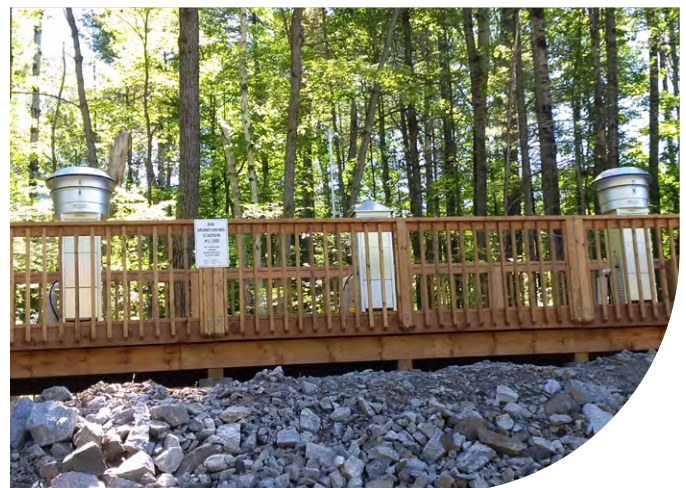
Dust monitors located at the NSDF site.
